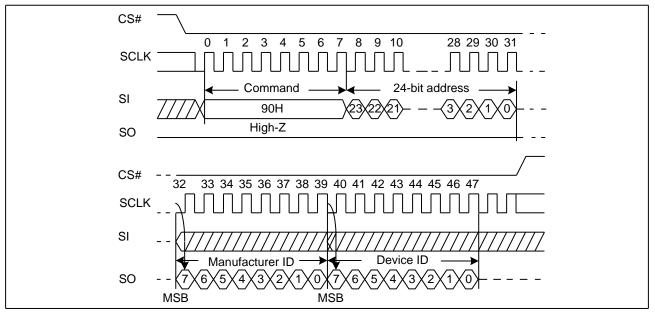
Figure 58 Read Manufacture ID/ Device ID Sequence Diagram
