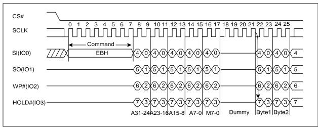
Figure 29 Quad I/O Fast Read Sequence Diagram (M5-4≠ (1, 0), ADS=1)
