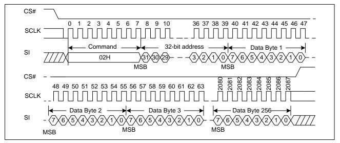
Figure 36 Page Program with 4-Byte Address Sequence Diagram (ADS=0 or ADS=1)
