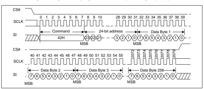
Figure 64 Program Security Registers command Sequence Diagram (ADS=0)
