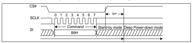
Figure 50 Deep Power-Down Sequence Diagram
