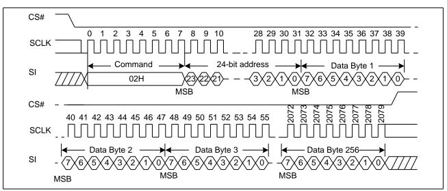
Figure 35 Page Program Sequence Diagram (ADS=1)
