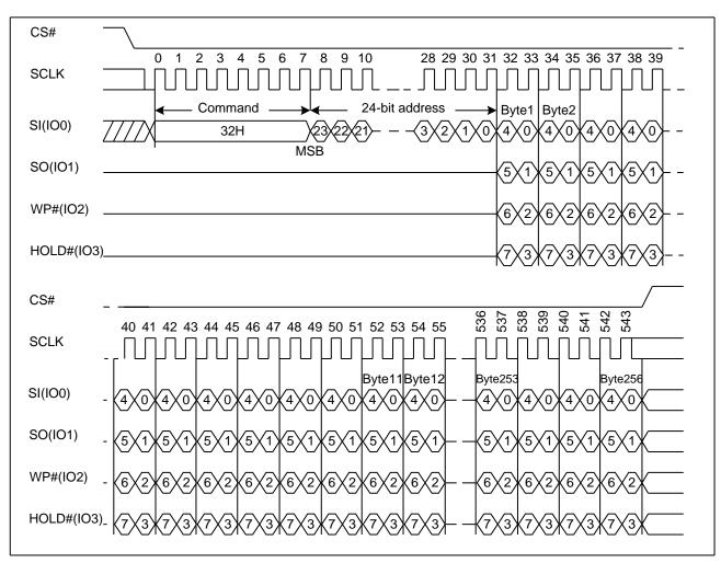
Figure 37 Quad Page Program Sequence Diagram (ADS=0)
