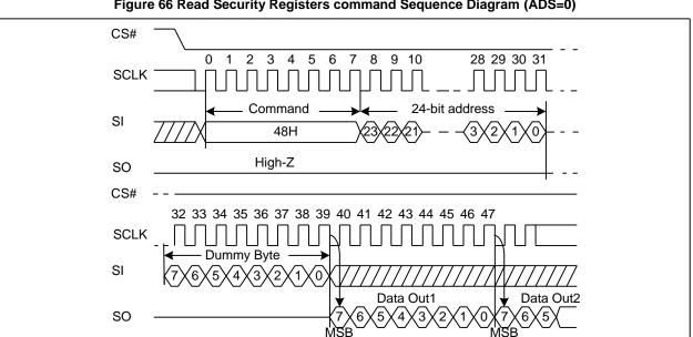
Figure 66 Read Security Registers command Sequence Diagram (ADS=0)
