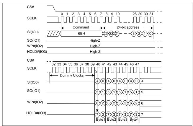
Figure 18 Quad Output Fast Read Sequence Diagram (ADS=0)
