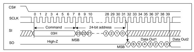
Figure 10 Read Data Bytes Sequence Diagram (ADS=1)
