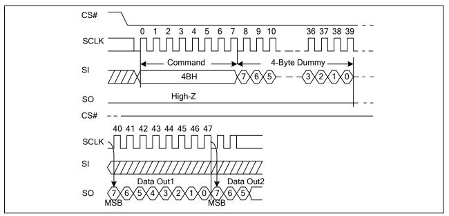
Figure 51 Read Unique ID Sequence Diagram (ADS=0)
