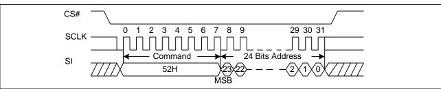
Figure 44 32KB Block Erase Sequence Diagram (ADS=1)
