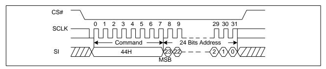
Figure 63 Erase Security Registers command Sequence Diagram (ADS=1)
