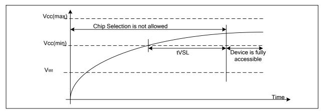
Table 24 Power-Up Timing and Write Inhibit Threshold
